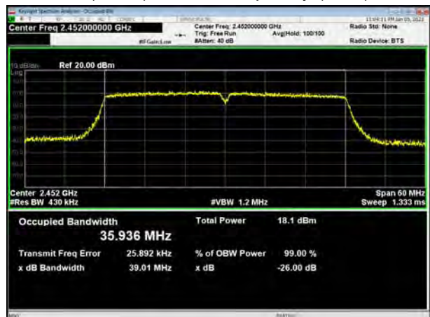
802.11n(HT40), Carrier frequency (MHz): 2452
