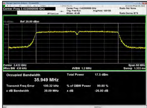
802.11n(HT40), Carrier frequency (MHz): 2437
