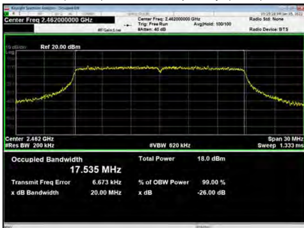
802.11n(HT20), Carrier frequency (MHz): 2462
