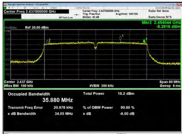
802.11n(HT40), Carrier frequency (MHz):2452
