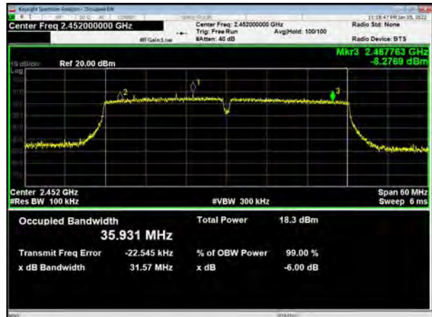
802.11n(HT40), Carrier frequency (MHz):2452
