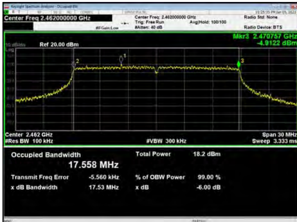
802.11n(HT20), Carrier frequency (MHz):2462
