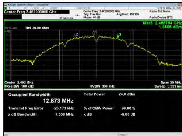
802.11b, Carrier frequency (MHz):2462
