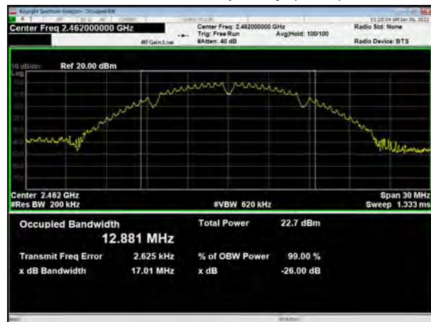
802.11b, Carrier frequency (MHz):2462
