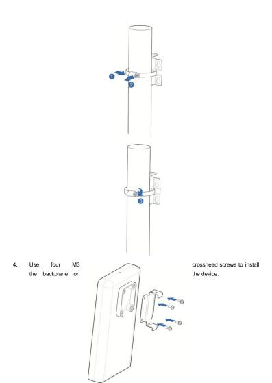
Firstly, fasten the backplane to the installed bracket through the upper and lower slots, and align the hole on the backplane with the hole on the bracket. Secondly, use one M3crosshead screw to install the MC7010CA on the bracket.
