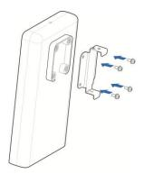
4. Firstly, fasten the backplane to the installed bracket through the upper and lower slots, and align the hole on thebackplane with the hole on the bracket.Secondly, use one M3crosshead screw to install the MC7010CA on the bracket.
