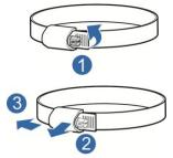
Pass the clamp through the U-shape groove on the bracket to install the bracket against the pole.
