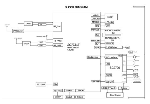
The equipment under test (EUT) is the transmitter of ZTE Blade L130, WCDMA (B2/B4/B5) and GSM(850//900/1800/1900) digital mobile phone. Single band 2.4GHz,support 802.11b/g/n ,Support WIFI and BT TDD operation and signle-antenna with intergrated TR-switch, and support GPS.
