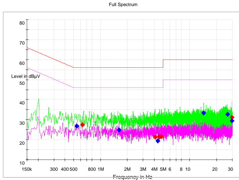
Pic5. Conducted emission N Line
