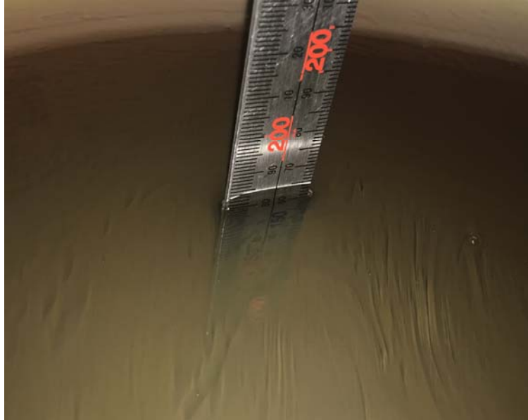
Liquid depth for SAR Measurement
