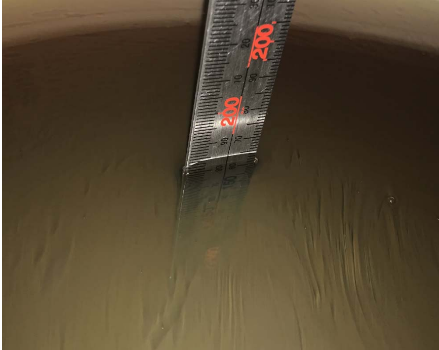
Liquid depth for SAR Measurement
