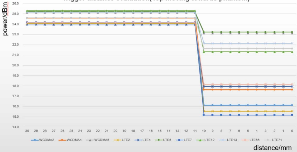
Trigger distance evaluation(Top moving towards phantom)
