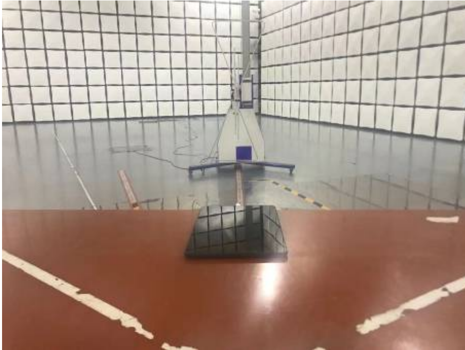
Radiated Emissions Test Setup (30-1000MHz)
