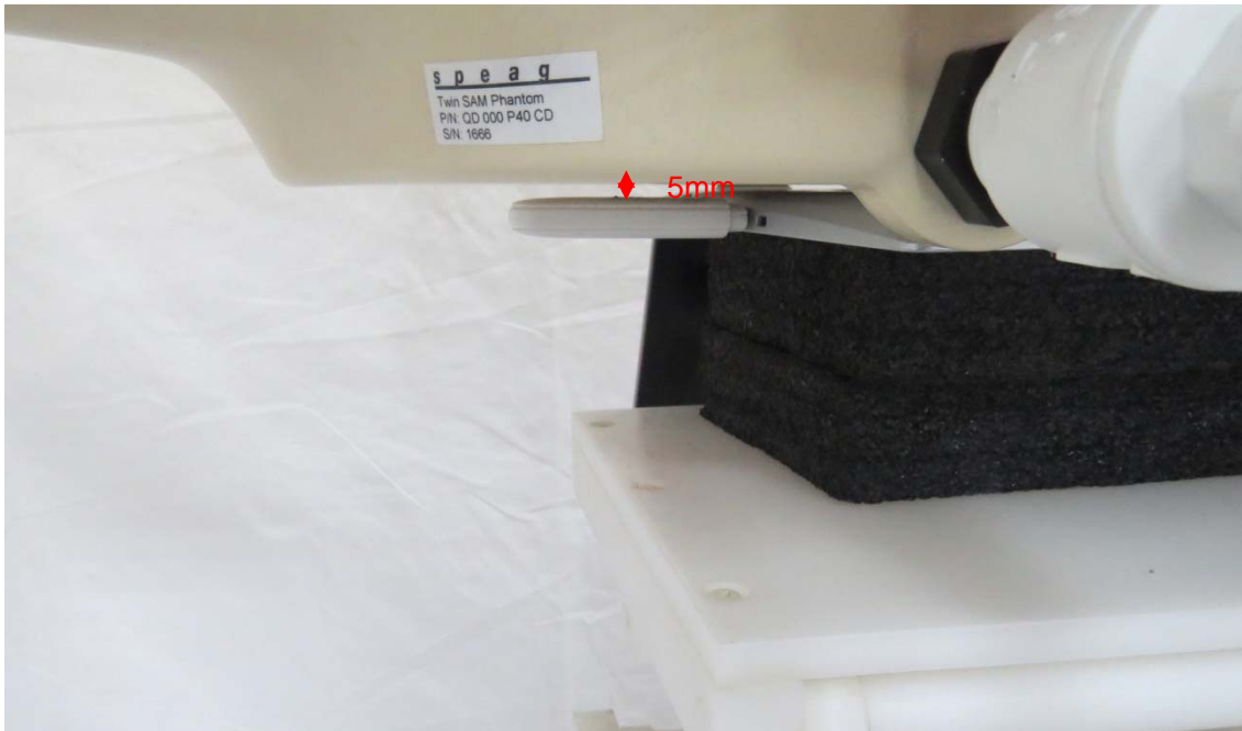
Picture 1: Back Side, the distance from handset to the bottom of the Phantom is 5mm
