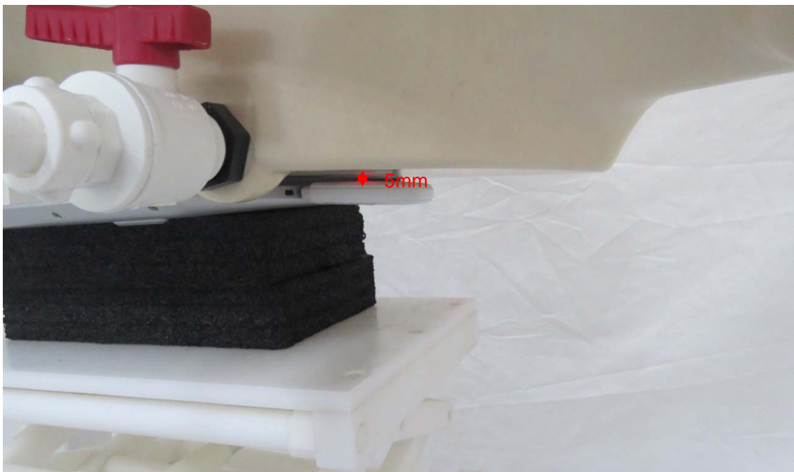
Picture 2: Front Side, the distance from handset to the bottom of the Phantom is 5mm
