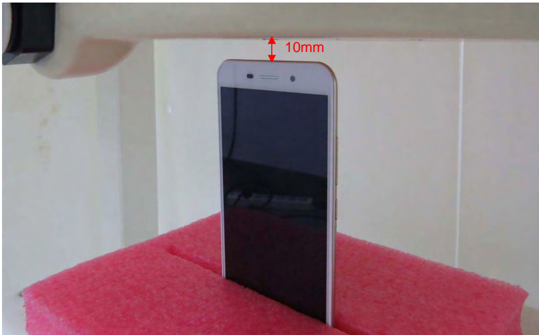
Picture 22: Top Side, the distance from handset to the bottom of the Phantom is 10mm
