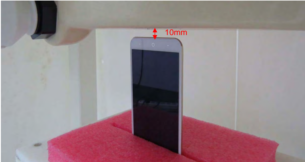
Picture 23: Bottom Side, the distance from handset to the bottom of the Phantom is 10mm
