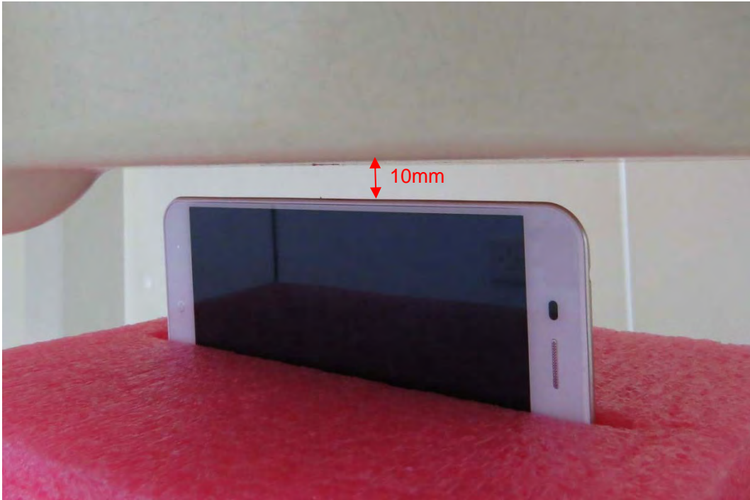
Picture 18: Left Side, the distance from handset to the bottom of the Phantom is 10mm
