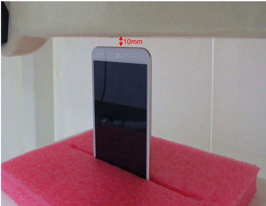
Picture 21: Bottom Side, the distance from handset to the bottom of the Phantom is 10mm
