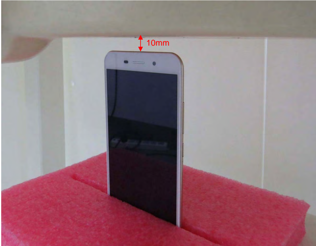
Picture 20: Top Side, the distance from handset to the bottom of the Phantom is 10mm
