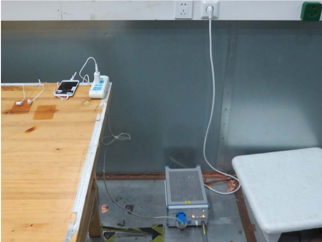
Picture 3 Conducted Emission Test Setup
