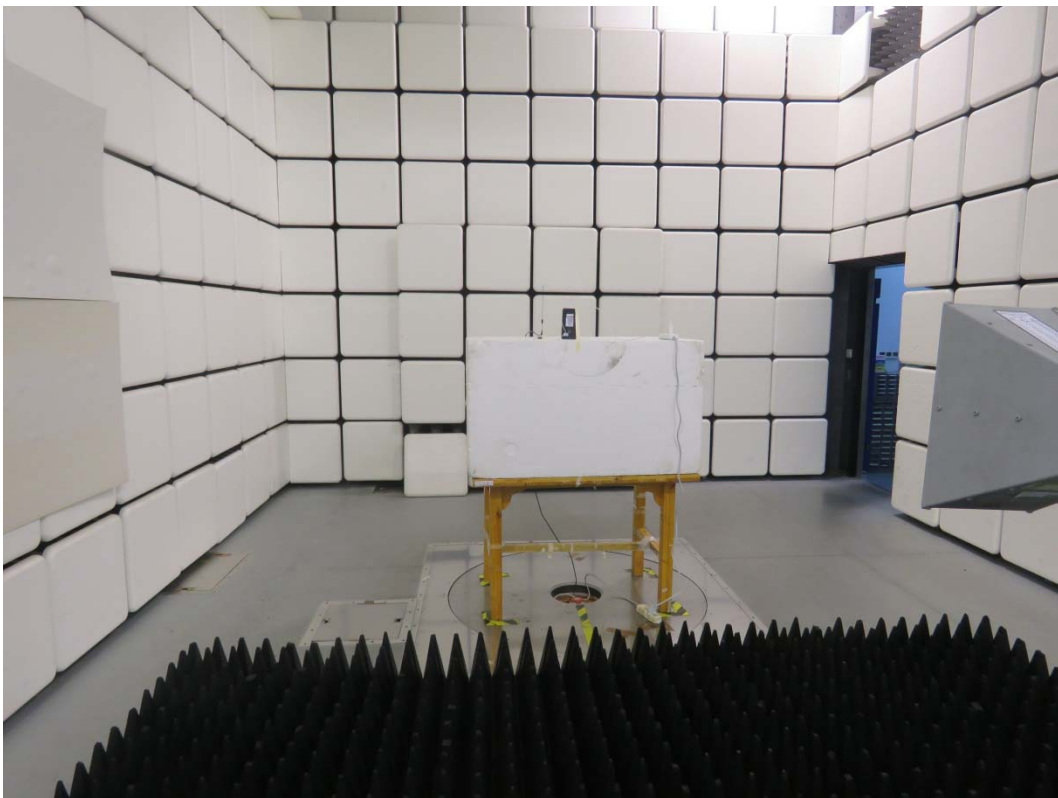
Picture 1: Radiated Spurious Emissions Test setup
