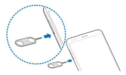
2. Pull out the card tray and place the nano-SIM card (right) /microSDXC card (left) facing down on the tray. Gently slide the card tray in until it clicks into place.
