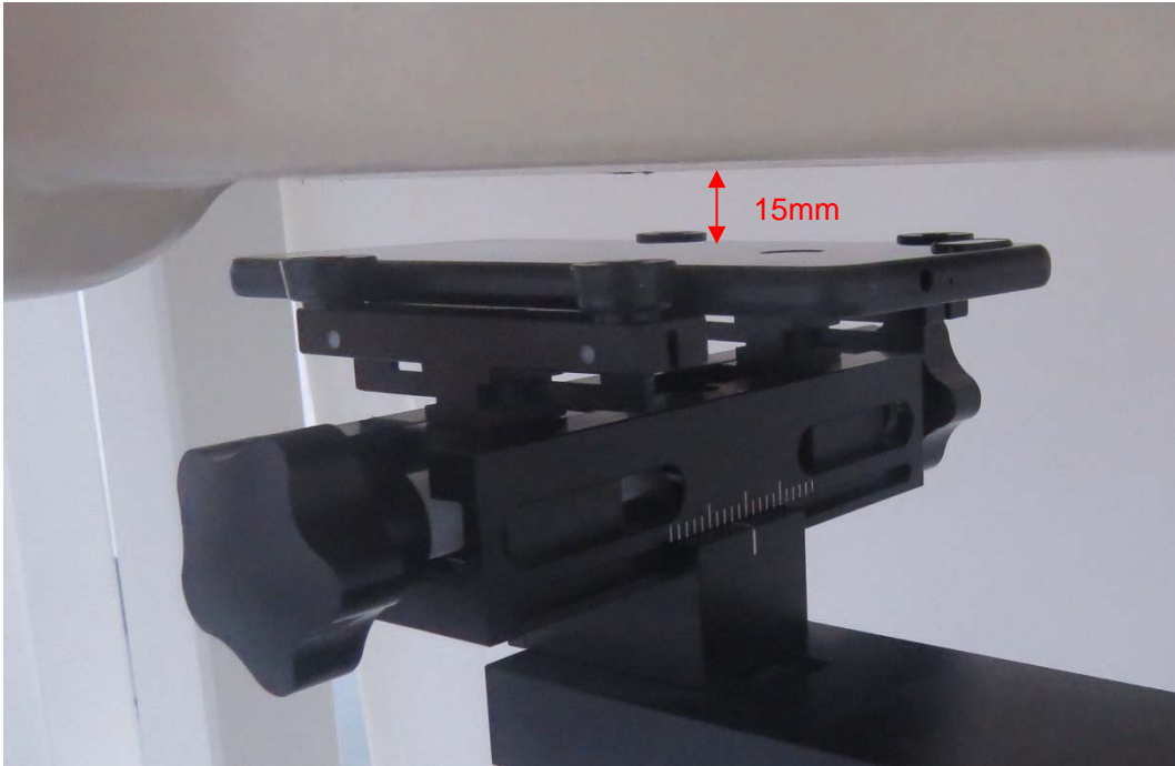
Picture 5: Back Side, the distance from handset to the bottom of the Phantom is 15mm
