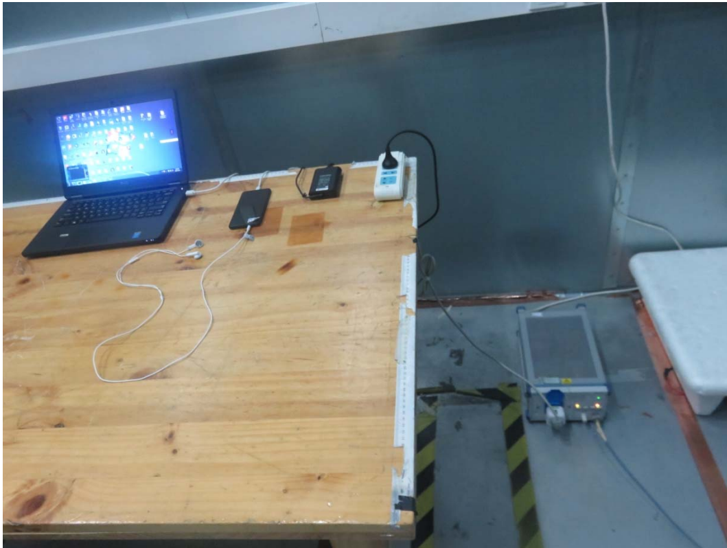
Picture 2 Conducted Emission Test Setup
