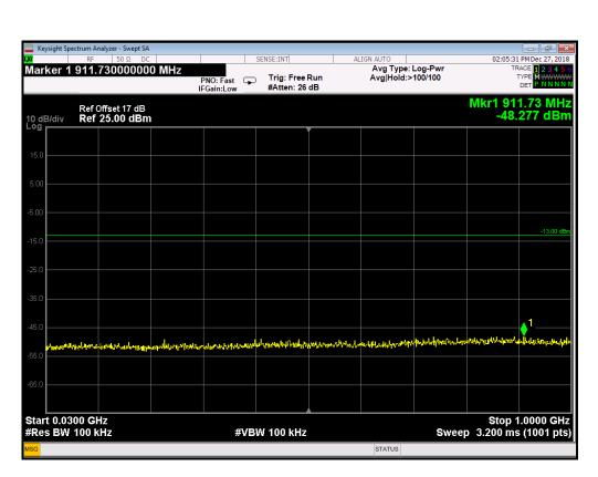
GSM 1900MHz Channel = 810, 30MHz to 1GHz
