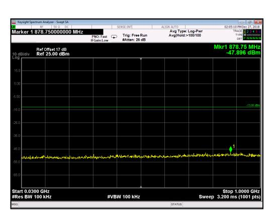
GSM 1900MHz Channel = 512, 30MHz to 1GHz
