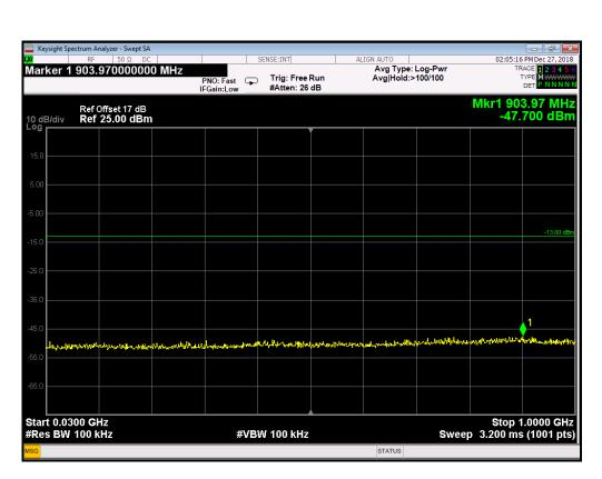
GSM 1900MHz Channel = 661, 30MHz to 1GHz
