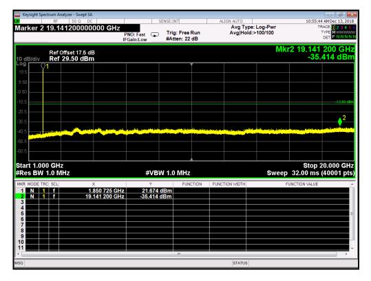
EDGE 1900MHz Channel = 512, 1GHz to 20GHz
