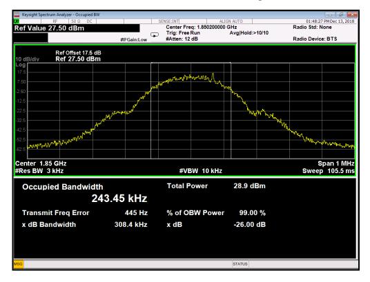
(Plot B1: GSM 1900MHz Channel = 512 Occupied bandwidth)
