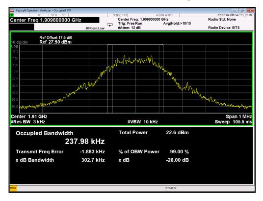
(Plot D3: EDGE 1900MHz Channel = 810 Occupied bandwidth)
