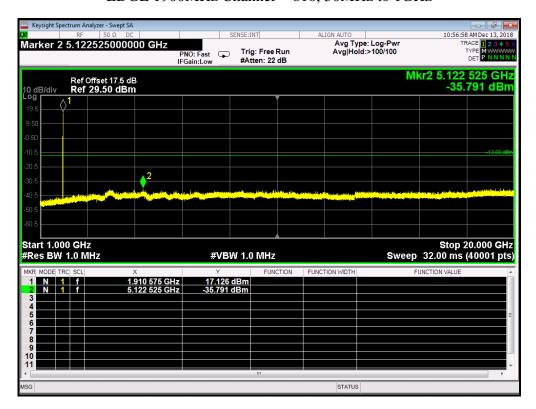
EDGE 1900MHz Channel = 810, 1GHz to 20GHz
