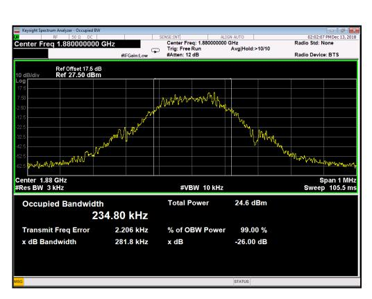
(Plot D2: EDGE 1900MHz Channel = 661 Occupied bandwidth)
