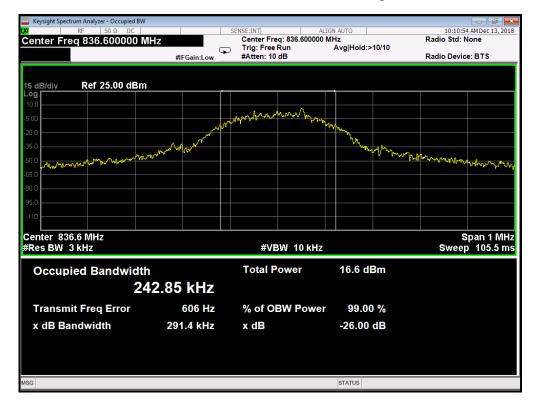
(Plot C2: EDGE 850MHz Channel = 190 Occupied bandwidth)
