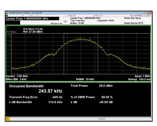
(Plot B2: GSM 1900MHz Channel = 661 Occupied bandwidth)
