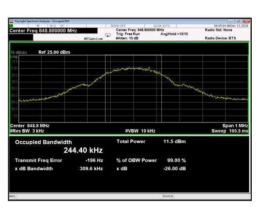
(Plot A3: GSM 850MHz Channel = 251 Occupied bandwidth)
