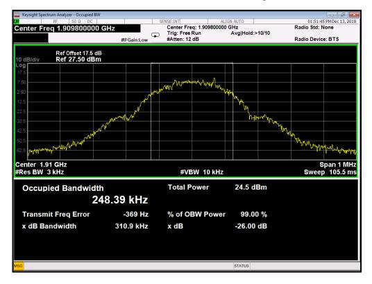
(Plot B3: GSM 1900MHz Channel = 810 Occupied bandwidth)
