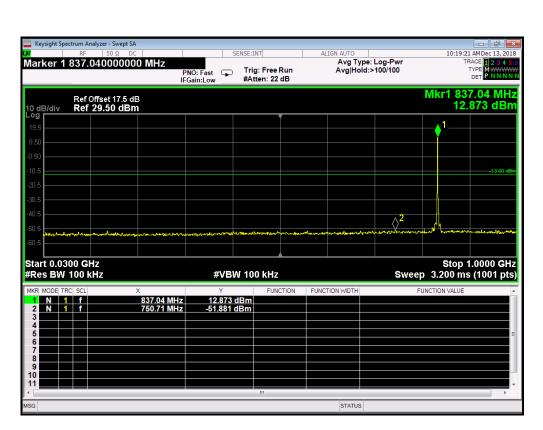
GSM 850MHz Channel = 190, 30MHz to 1GHz
