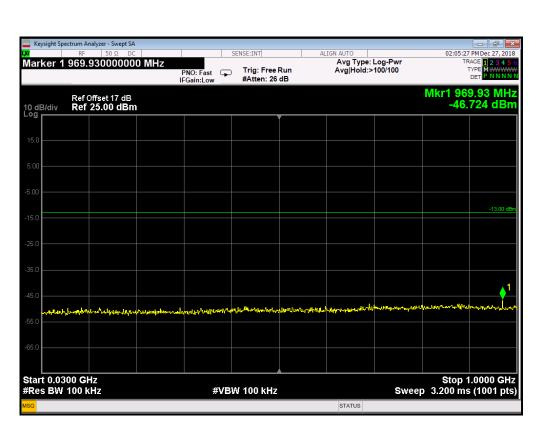
EDGE 1900MHz Channel = 810, 30MHz to 1GHz
