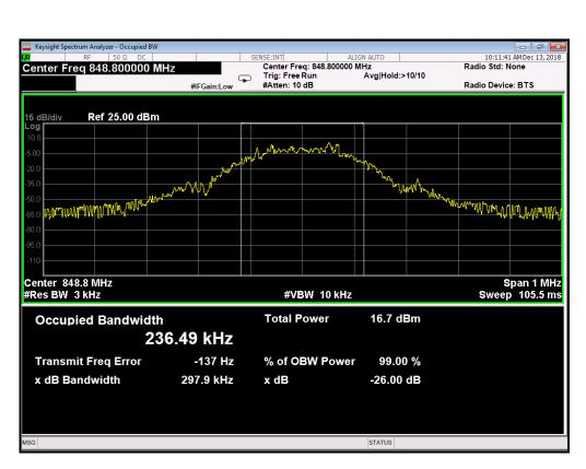
(Plot C3: EDGE 850MHz Channel = 251 Occupied bandwidth)
