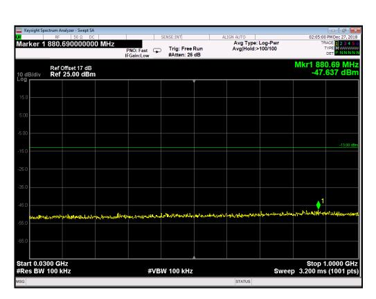
EDGE 1900MHz Channel = 661, 30MHz to 1GHz
