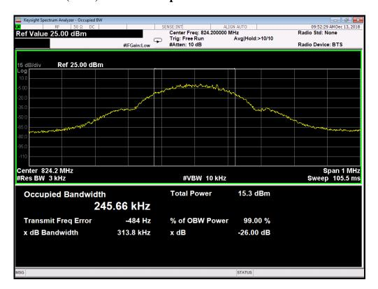
(Plot A1: GSM 850MHz Channel = 128 Occupied bandwidth)
