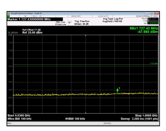
EDGE 1900MHz Channel = 512, 30MHz to 1GHz
