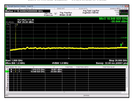
GSM 1900MHz Channel = 810, 1GHz to 20GHz
