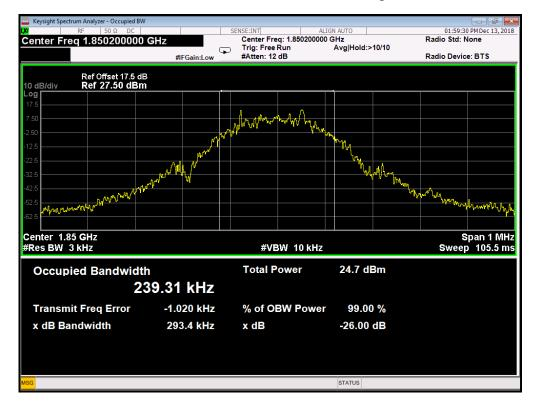
(Plot D1: EDGE 1900MHz Channel = 512 Occupied bandwidth)
