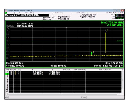
GSM 850MHz Channel = 251, 30MHz to 1GHz
