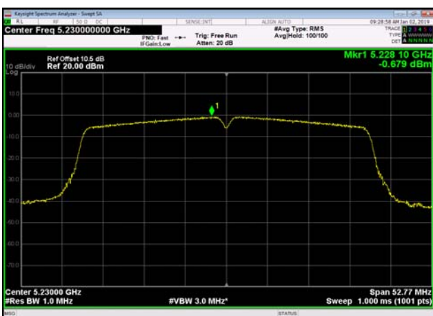
U-NII-1 Power spectral density-802.11 n(40MHz),5230MHz
