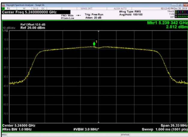
U-NII-1 Power spectral density-802.11 ac(20MHz),5240MHz
