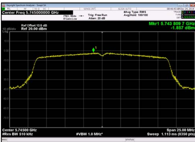
U-NII-3 Power spectral density-802.11 ac(20MHz),5745MHz
