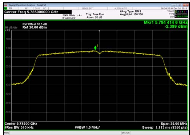
U-NII-3 Power spectral density-802.11 ac(20MHz),5785MHz
