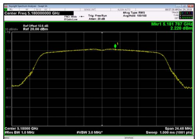
U-NII-1 Power spectral density-802.11 a(20MHz),5180MHz
