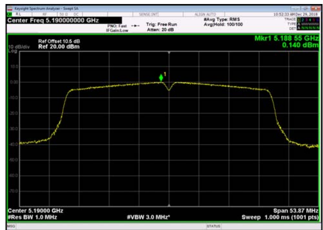
U-NII-1 Power spectral density-802.11 ac(40MHz),5190MHz
