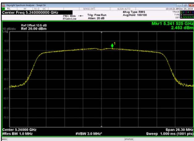
U-NII-1 Power spectral density-802.11 n(40MHz),5230MHz
