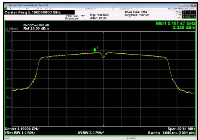
U-NII-1 Power spectral density-802.11 a(20MHz),5180MHz
