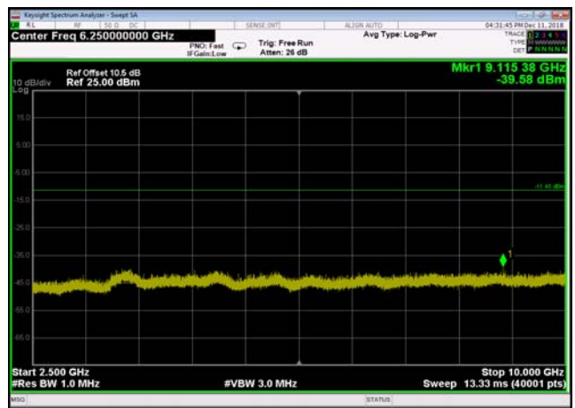
Conducted Emission: pi/4DQPSK,2441,2DH5 ,Band Edge HoppingOFF
