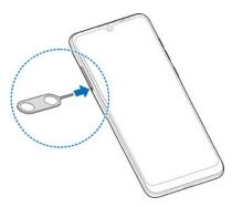
Pull out the card tray and place a nano-SIM card and a microSDXC card (optional) on the tray, as shown. Carefully slide the tray back into place.
