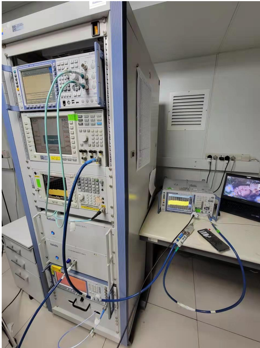
RF Conducted Test setup (GSM/WCDMA/LTE)
