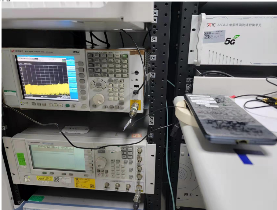
RF Conducted Test setup (BT/WIFI)
