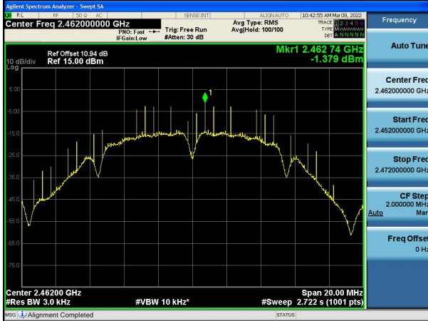
Test Mode:802.11b 2462MHz Chain0
