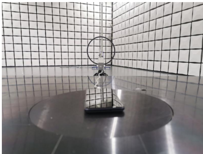
Conducted Emissions Test Setup (with charger)
