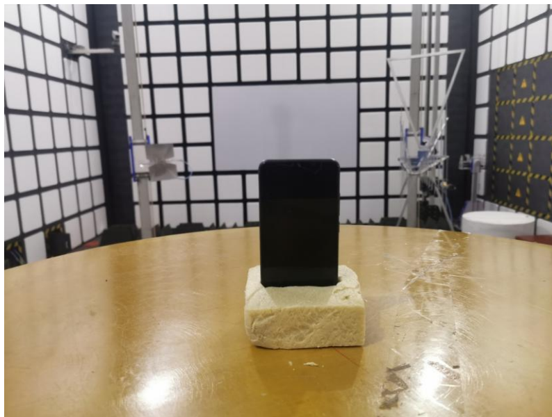
Spurious Radiated Emissions Test setup
