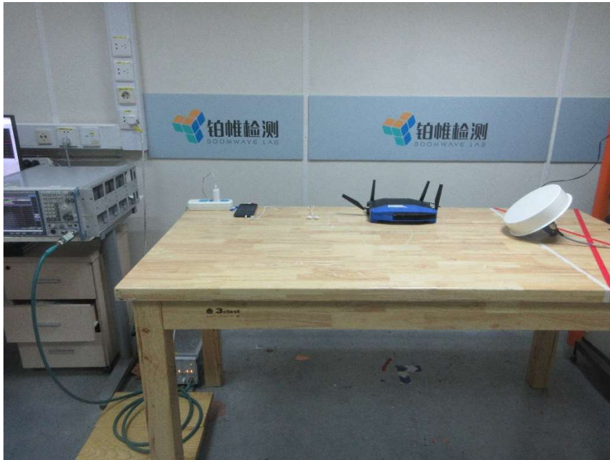
Conducted Emission 150kHz-30MHz (Front view) – Mode 2
