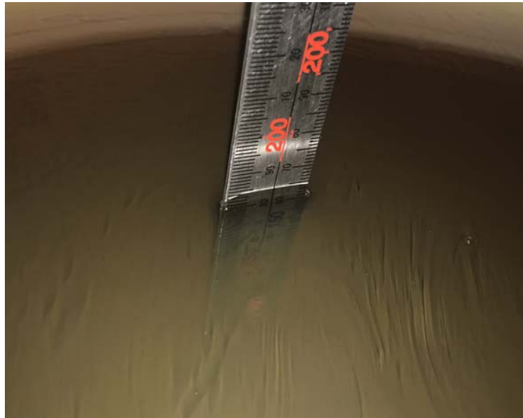
Liquid depth for SAR Measurement
