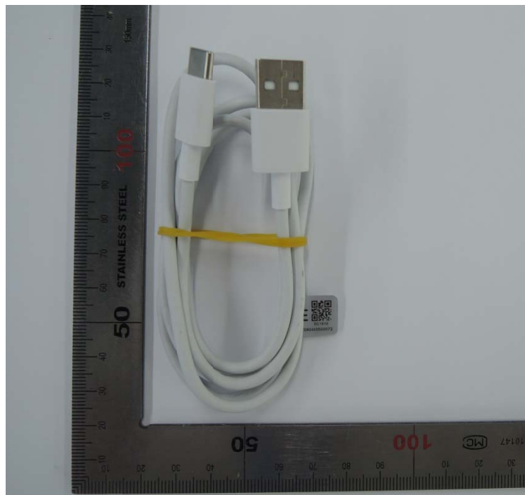
USB Cable A (Model Number: USB-TC20-W-100-M-L-HF Manufacture: Luxshare-ICT Co., Ltd)
