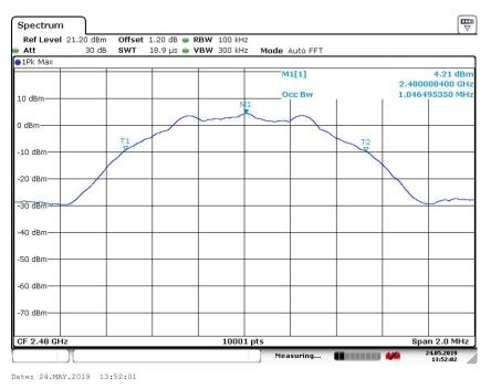
Carrier frequency (MHz): 2480 Channel No.:39 Modulation type: GFSK (LE 1Mbps)
