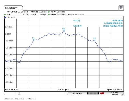
Carrier frequency (MHz): 2480 Channel No.:39 Modulation type: GFSK (LE 2Mbps)
