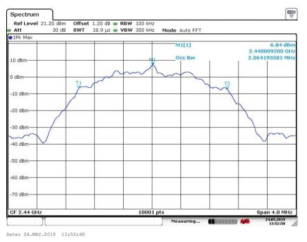
Carrier frequency (MHz): 2440 Channel No.:19 Modulation type: GFSK (LE 2Mbps)
