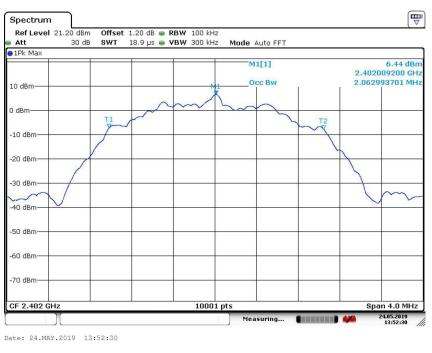
Carrier frequency (MHz): 2402 Channel No.:0 Modulation type: GFSK (LE 2Mbps)
