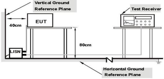
For the actual test configuration, please refer to the attached file (Test Setup Photo).
