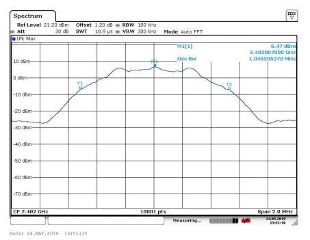
Carrier frequency (MHz): 2402 Channel No.:0 Modulation type: GFSK (LE 1Mbps)
