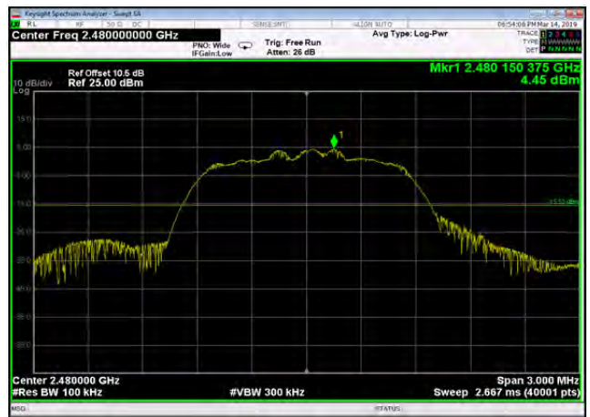
Conducted Emission: DQPSK,2480,2DH5 ,Reference Level
