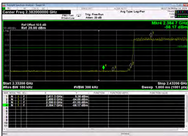
Conducted Emission: 8DPSK,2402,3DH5 ,Band Edge
