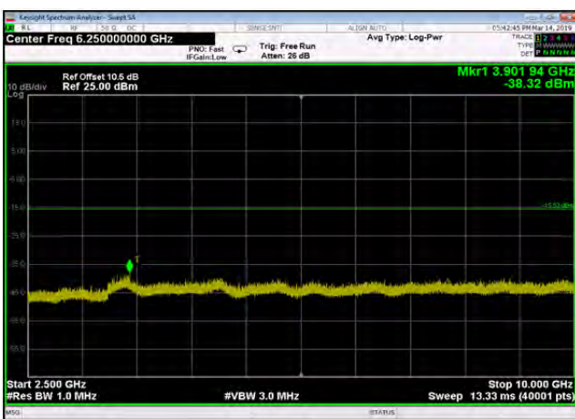
Conducted Emission: DQPSK,2402,2DH5 ,2500MHz~10000MHz
