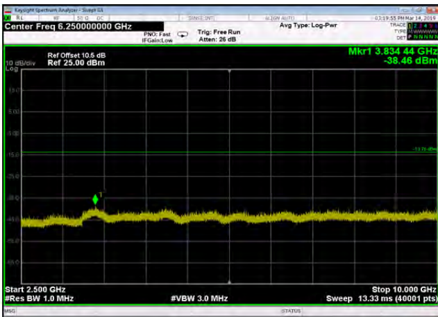
Conducted Emission: GFSK,2441,DH5 ,Band Edge HoppingOFF
