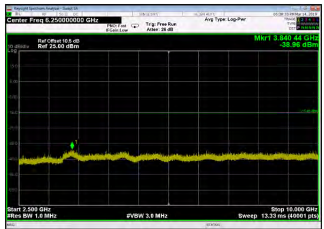
Conducted Emission: DQPSK,2441,2DH5 ,Band Edge HoppingOFF
