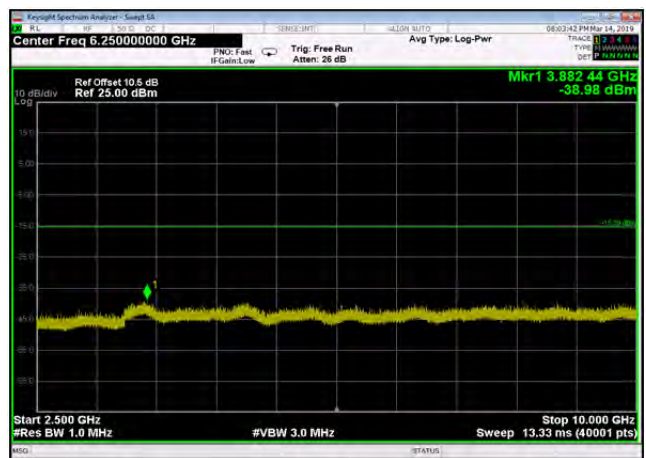
Conducted Emission: 8DPSK,2480,3DH5 ,2500MHz~10000MHz
