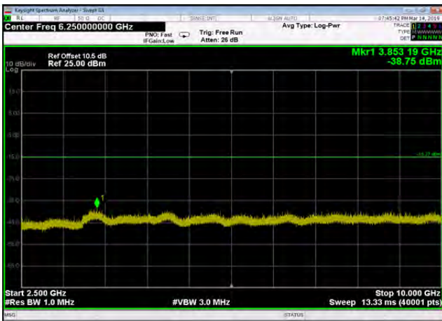
Conducted Emission: 8DPSK,2441,3DH5 ,Band Edge HoppingOFF
