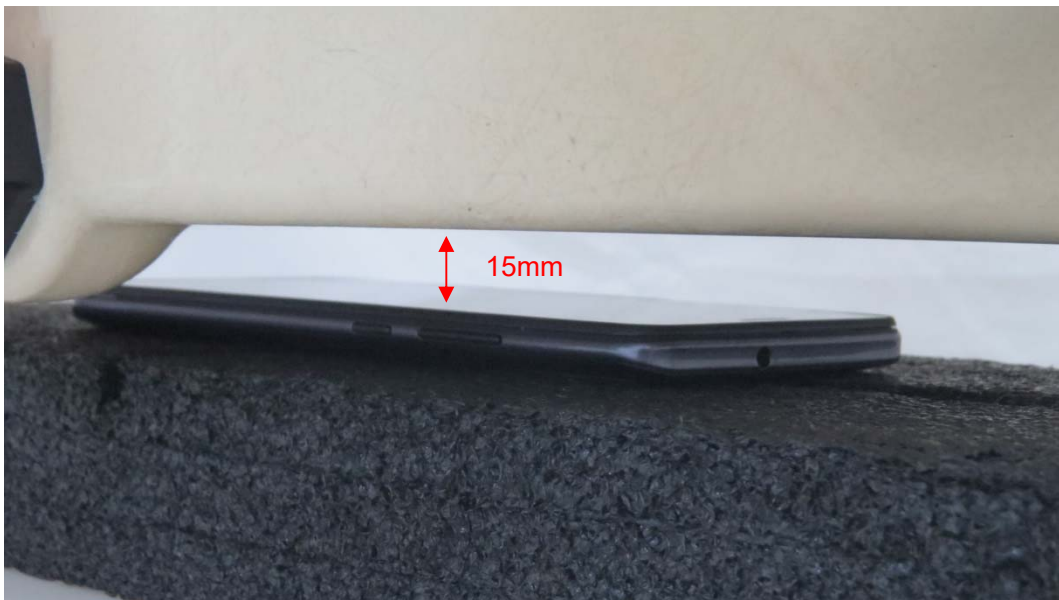
Picture 6: Front Side, the distance from handset to the bottom of the Phantom is 15mm
