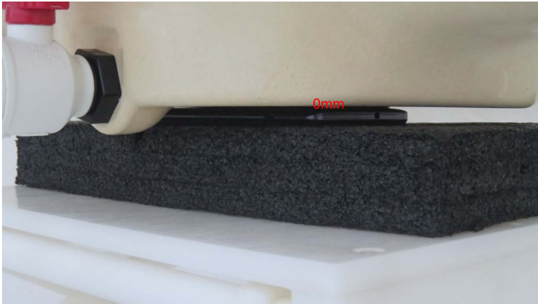
Picture 13: Back Side, the distance from handset to the bottom of the Phantom is 0mm
