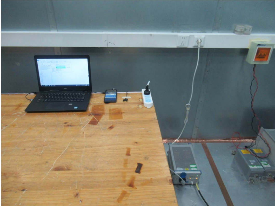
Picture 1: Conducted Emissions Test Setup
