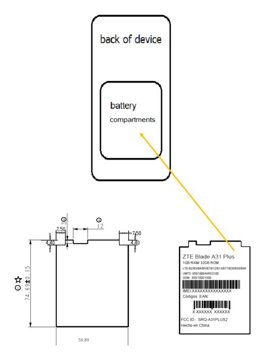
The label is on the device which is under the battery.
