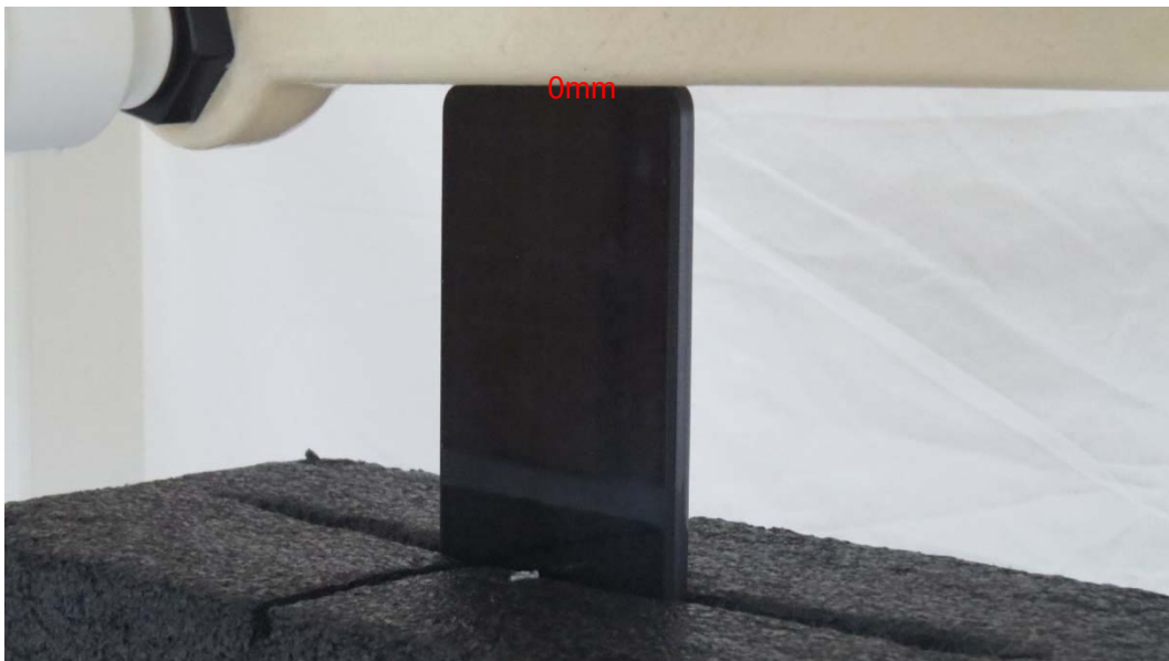
Picture 14: Bottom Edge, the distance from handset to the bottom of the Phantom is 0mm
