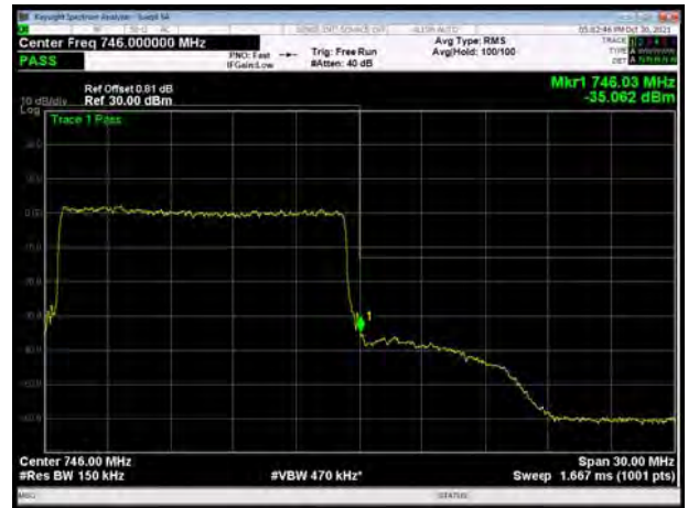
LTE Band 28 64QAM 15MHz CH-High, 100%RB
