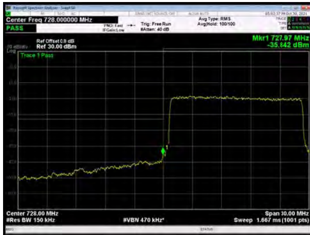
LTE Band 28 64QAM 15MHz CH-Low, 100%RB
