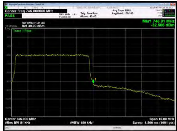
LTE Band 28 16QAM 5MHz CH-High, 100%RB
