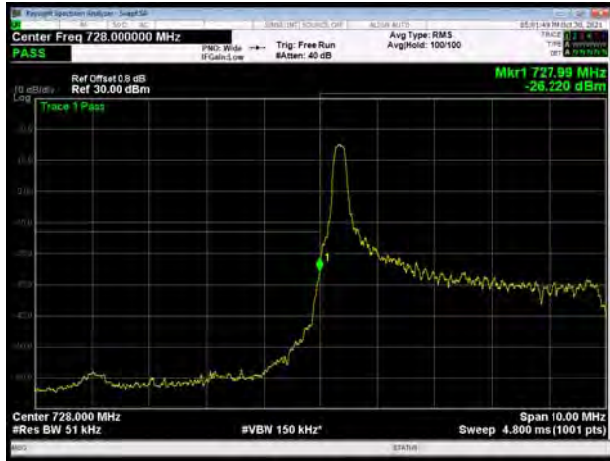
LTE Band 28 64QAM 5MHz CH-Low, 100%RB
