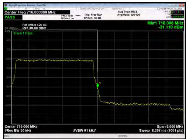
LTE Band 28 QPSK 5MHz CH-High, 1 RB
