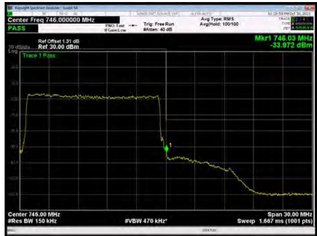
LTE Band 28 16QAM 3MHz CH-High, 1 RB
