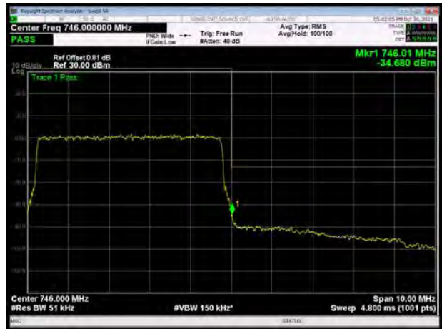
LTE Band 28 64QAM 10MHz CH-High, 1 RB
