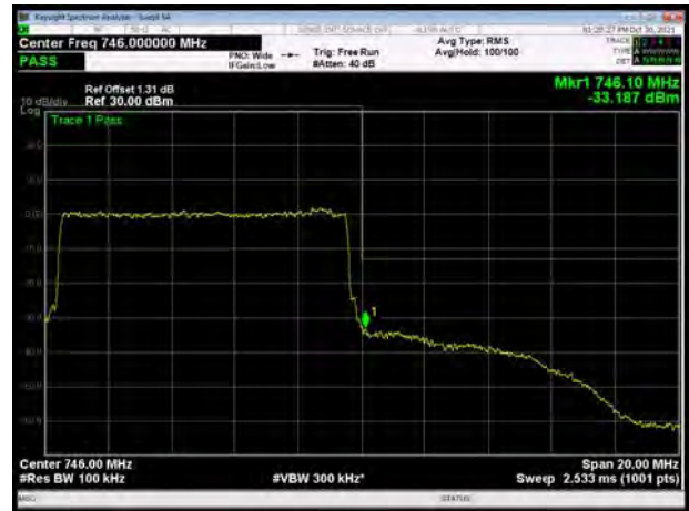
LTE Band 28 16QAM 15MHz CH-High, 1 RB
