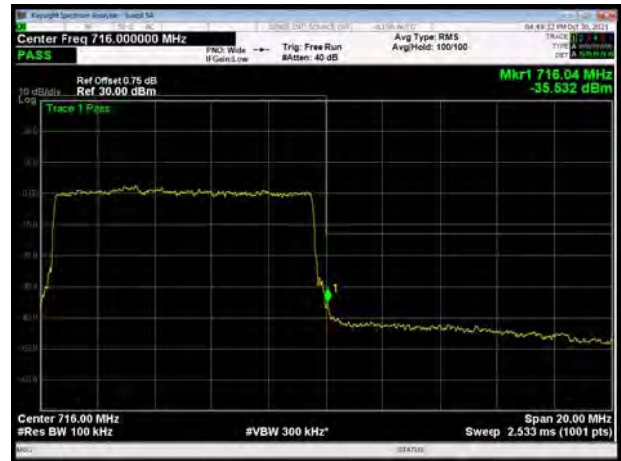
LTE Band 28 64QAM 10MHz CH-High, 100%RB
