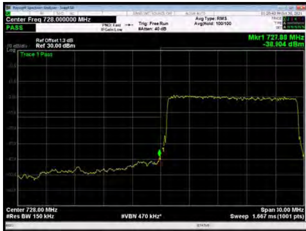
LTE Band 28 16QAM 3MHz CH-Low, 1 RB
