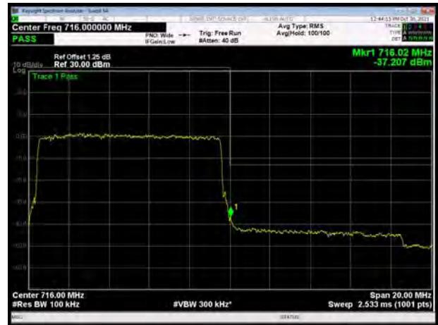
LTE Band 28 QPSK 10MHz CH-High, 100%RB
