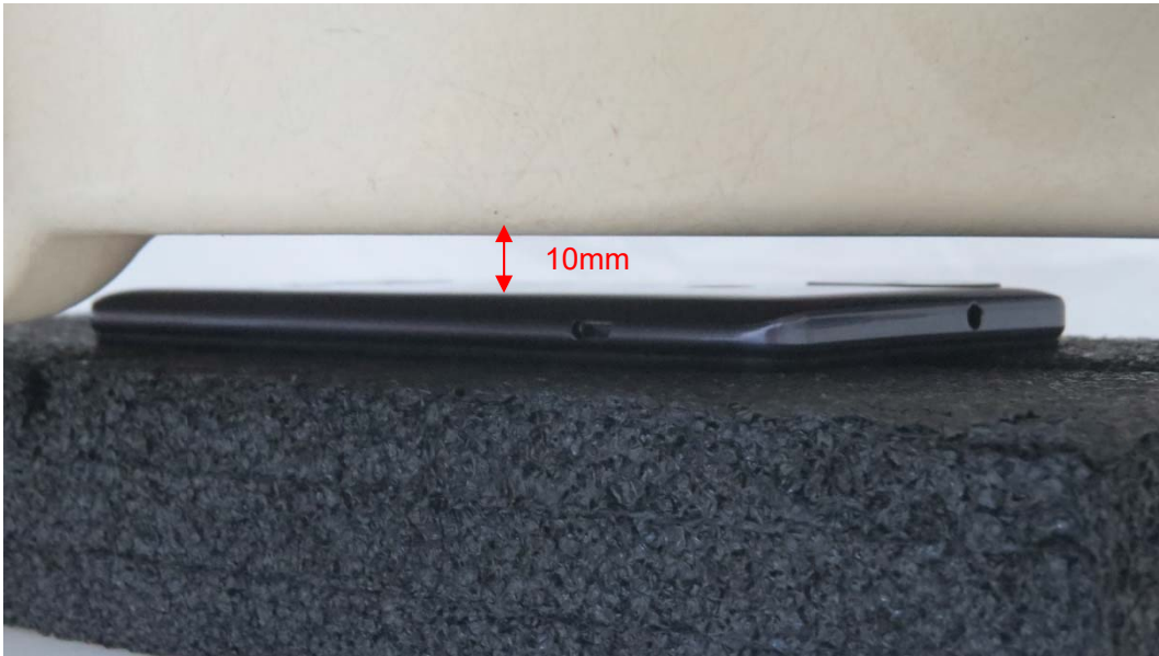
Picture 7: Back Side, the distance from handset to the bottom of the Phantom is 10mm
