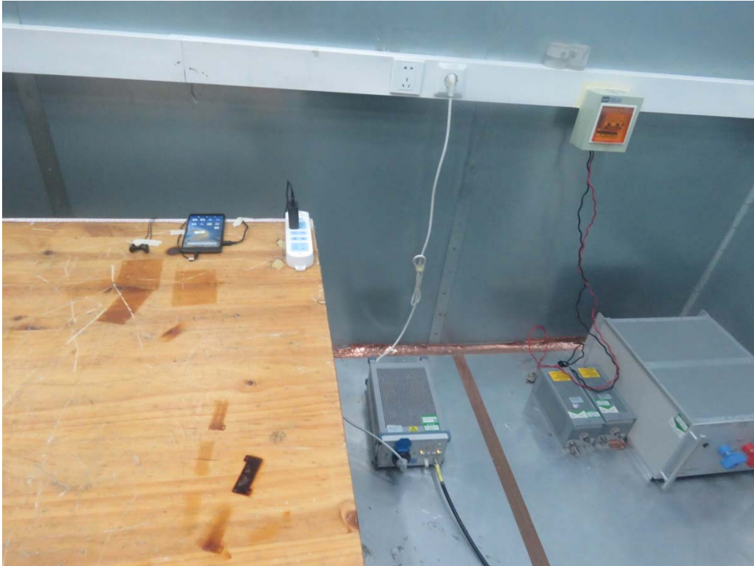
Picture 2 Conducted Emission Test Setup
