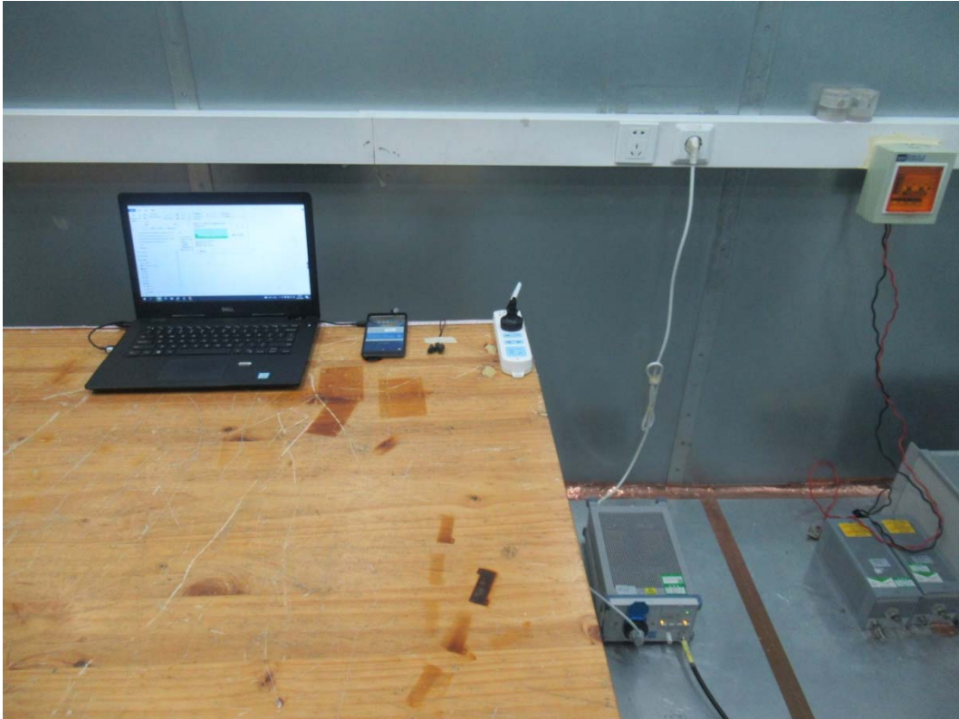
Picture 1: Conducted Emissions Test Setup
