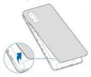
Insert the nano-SIM card into the right card slot, and insert the microSDXC card (optional) into the left card slot.
