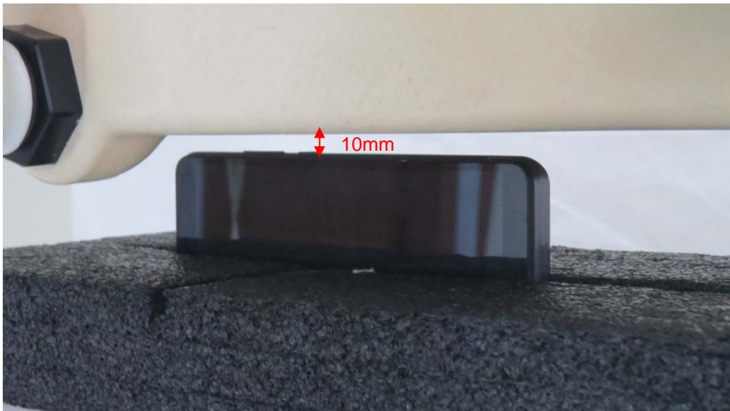
Picture 10: Right Side, the distance from handset to the bottom of the Phantom is 10mm
