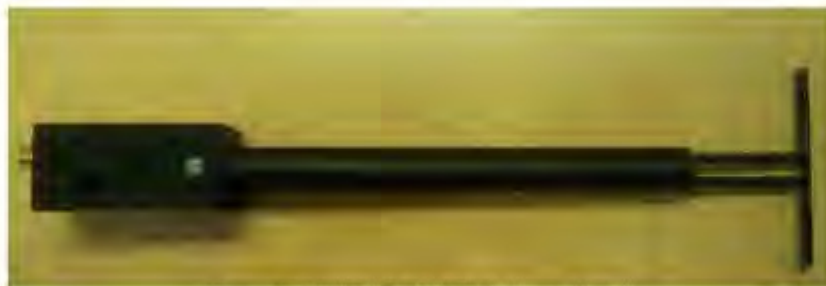
Figure 1 – MVG COMOSAR Validation Dipole
