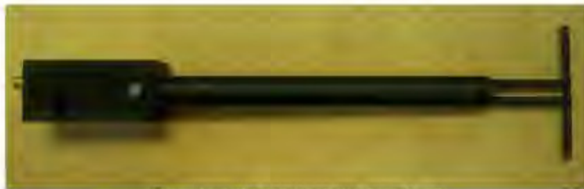
Figure 1 – MVG COMOSAR Validation Dipole
