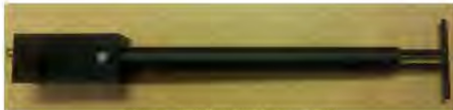
Figure 1 – MVG COMOSAR Validation Dipole
