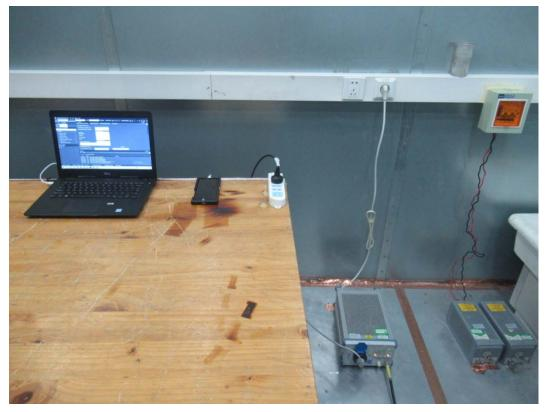
Picture 2: Conducted Emissions Test Setup
