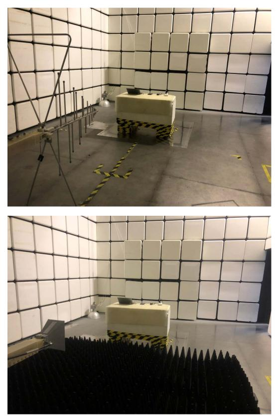
Picture 1: Radiated Emission Test Setup
