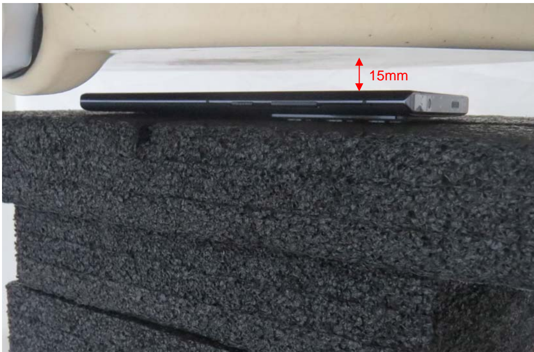
Picture 6: Front Side, the distance from handset to the bottom of the Phantom is 15mm
