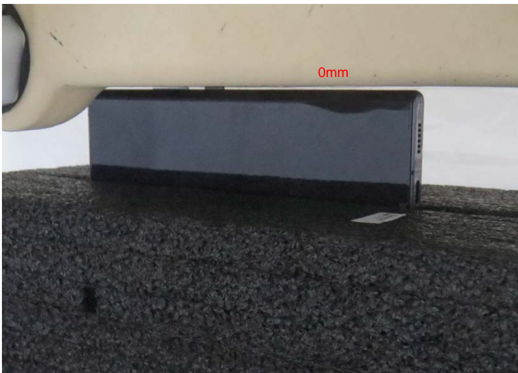
Picture 16: Right Edge, the distance from handset to the bottom of the Phantom is 0mm
