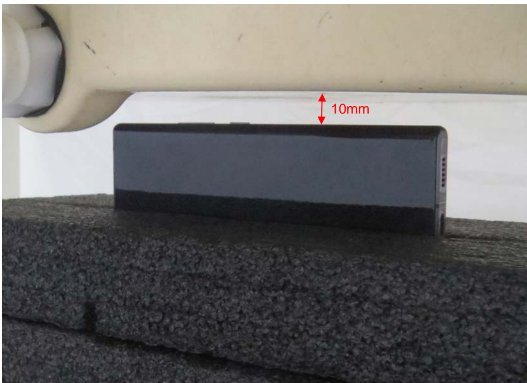
Picture 10: Right Edge, the distance from handset to the bottom of the Phantom is 10mm
