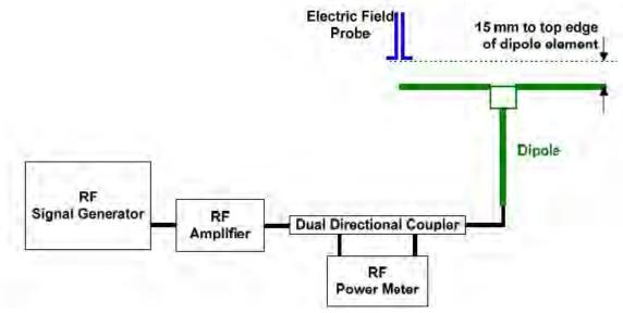
Figure 5 Dipole Validation Setup
