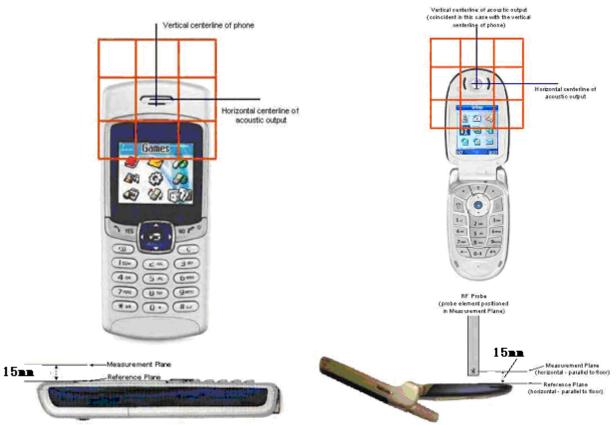
Figure 4 WD reference and plane for RF emission measurements
