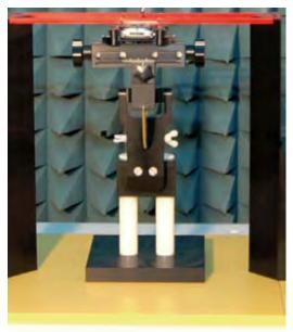
Figure 3 HAC Phantom & Device Holder
