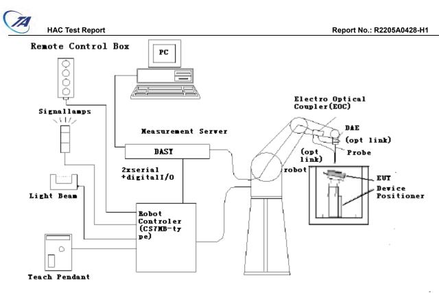
Figure 1 HAC Test Measurement Set-up
