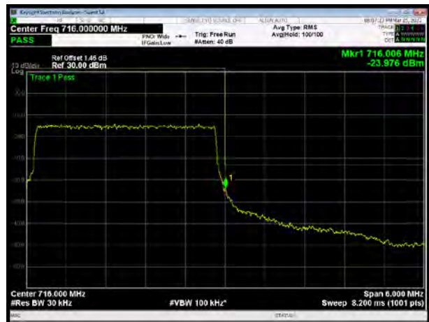
LTE Band 12 QPSK 5MHz CH-High, 1 RB
