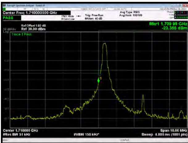
LTE Band 66 16QAM 5MHz CH-Low, 100%RB
