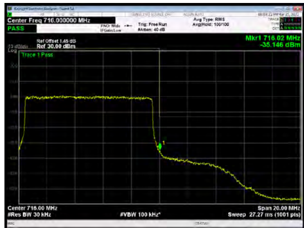
LTE Band 12 16QAM 1.4MHz CH-High, 1 RB
