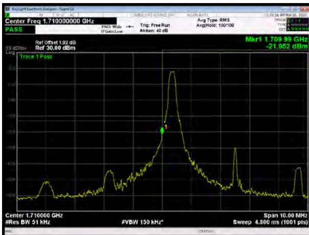
LTE Band 4 16QAM 5MHz CH-Low, 100%RB
