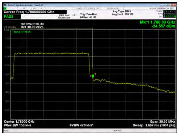
LTE Band 66 QPSK 20MHz CH-High, 1 RB
