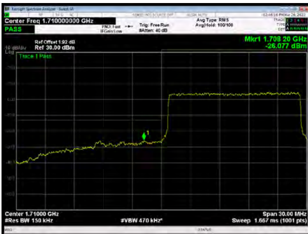
LTE Band 66 QPSK 20MHz CH-Low, 1 RB
