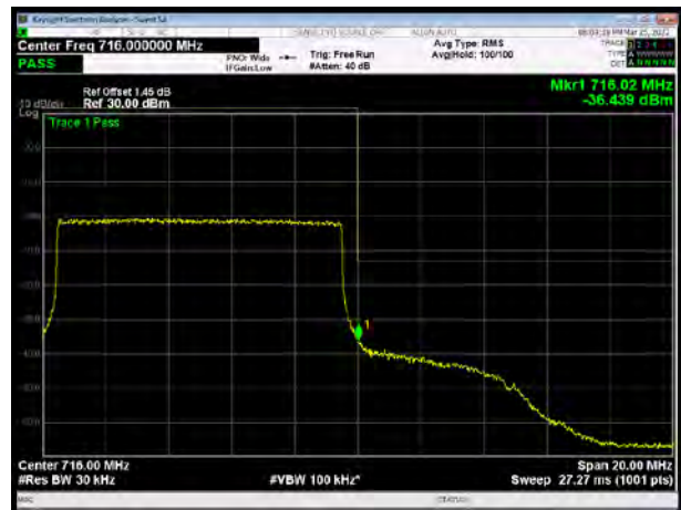
LTE Band 12 64QAM 1.4MHz CH-High, 1 RB
