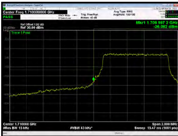
LTE Band 4 16QAM 3MHz CH-Low, 1 RB
