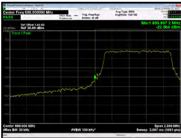
LTE Band 12 16QAM 3MHz CH-Low, 1 RB
