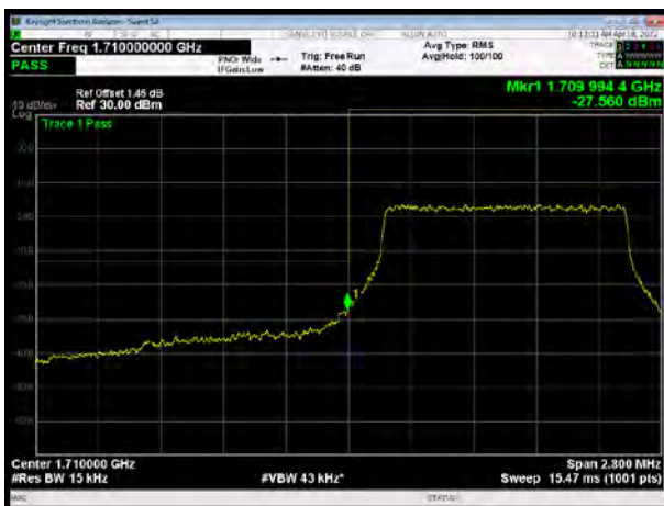
LTE Band 4 64QAM 3MHz CH-Low, 1 RB
