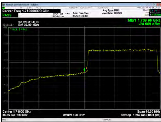
LTE Band 66 64QAM 20MHz CH-Low, 100%RB
