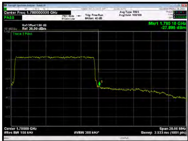
LTE Band 66 16QAM 15MHz CH-High, 1 RB
