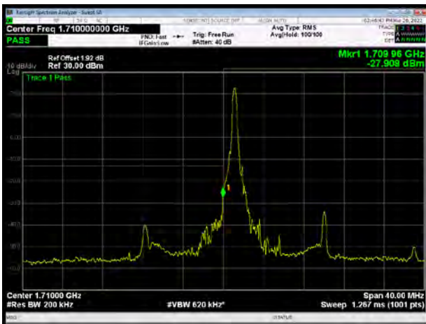
LTE Band 66 QPSK 20MHz CH-Low, 100%RB
