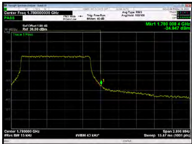
LTE Band 66 QPSK 3MHz CH-High, 1 RB
