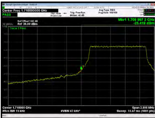
LTE Band 66 QPSK 3MHz CH-Low, 1 RB
