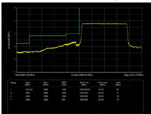
LTE Band 7 QPSK 15MHz CH-Low, 100%RB
