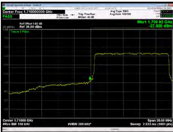
LTE Band 66 16QAM 15MHz CH-Low, 1 RB
