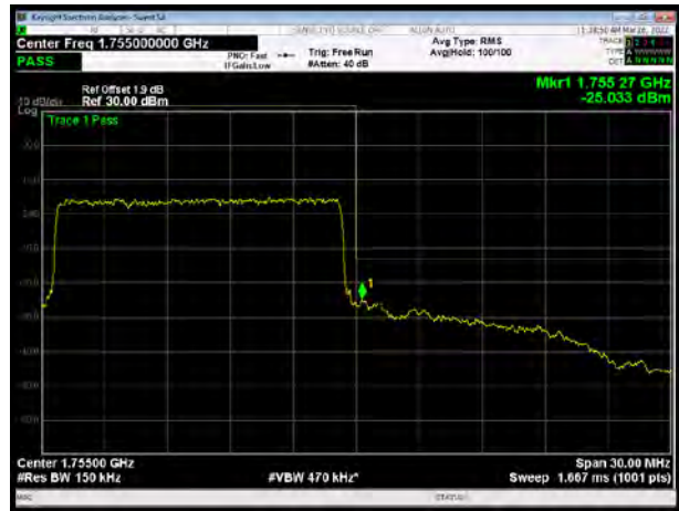
LTE Band 4 QPSK 20MHz CH-High, 1 RB
