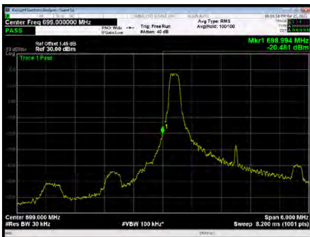
LTE Band 12 QPSK 3MHz CH-Low, 1 RB
