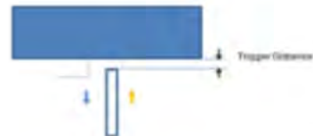
Picture : Proximity sensor triggering distances assessment(Bottom edge)
