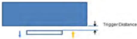
Picture : Proximity sensor triggering distances assessment(Back side)
