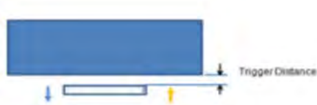
Picture : Proximity sensor triggering distances assessment(Back side)
