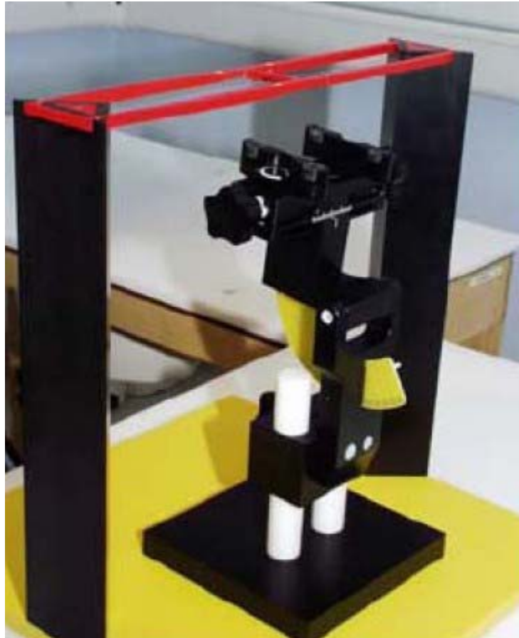
Figure 7 T-coil Phantom & Device Holder
