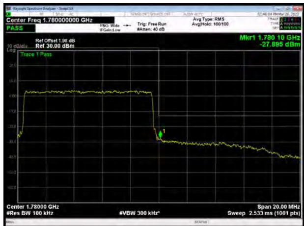
LTE Band 66 16QAM 15MHz CH-High, 1 RB
