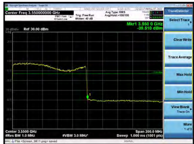
NR n77 subset 1 256QAM 100MHz CH-High 1RB
