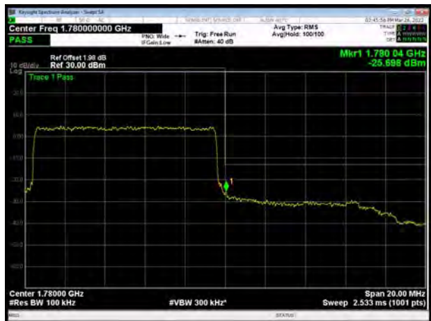
LTE Band 66 QPSK 15MHz CH-High, 1 RB
