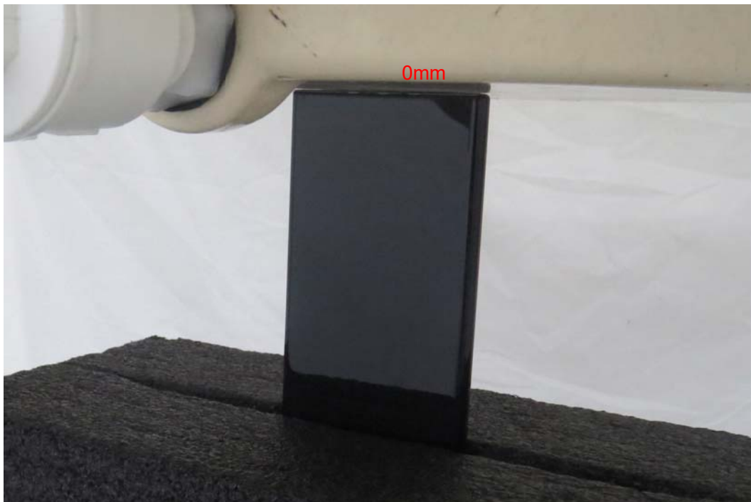
Picture 18: Bottom Edge, the distance from handset to the bottom of the Phantom is 0mm
