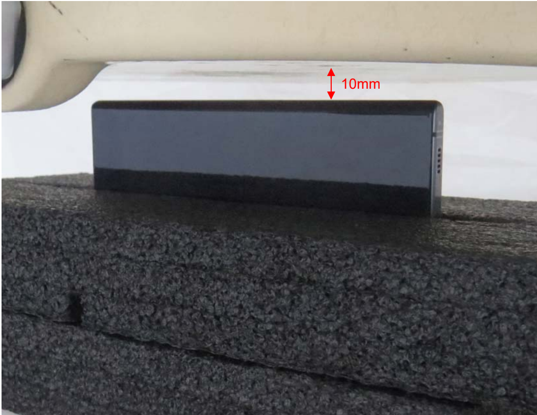
Picture 9: Left Edge, the distance from handset to the bottom of the Phantom is 10mm
