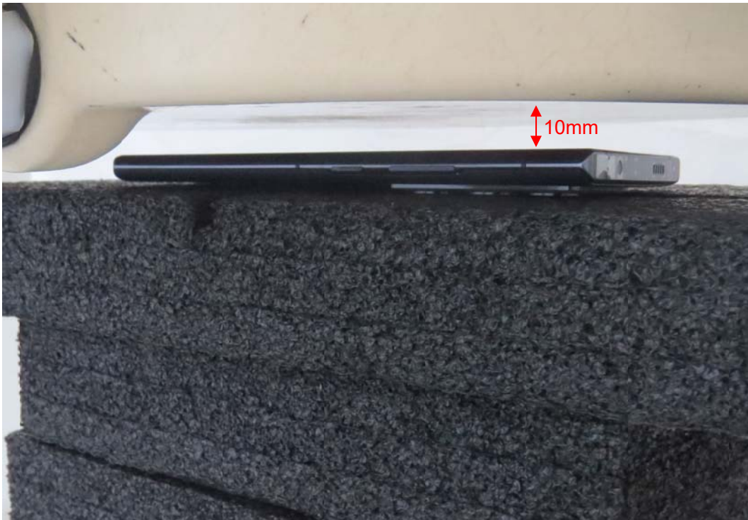
Picture 8: Front Side, the distance from handset to the bottom of the Phantom is 10mm
