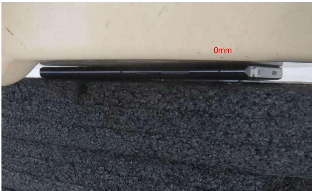
Picture 14: Front Side, the distance from handset to the bottom of the Phantom is 0mm
