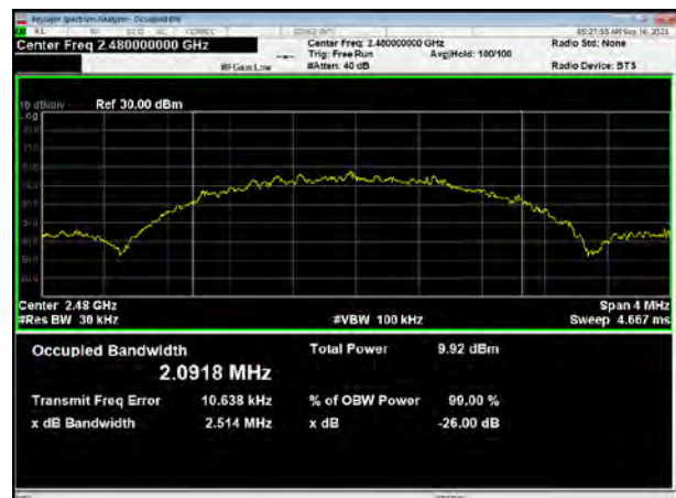
Bluetooth LE (2M) Carrier frequency (MHz): 2480
