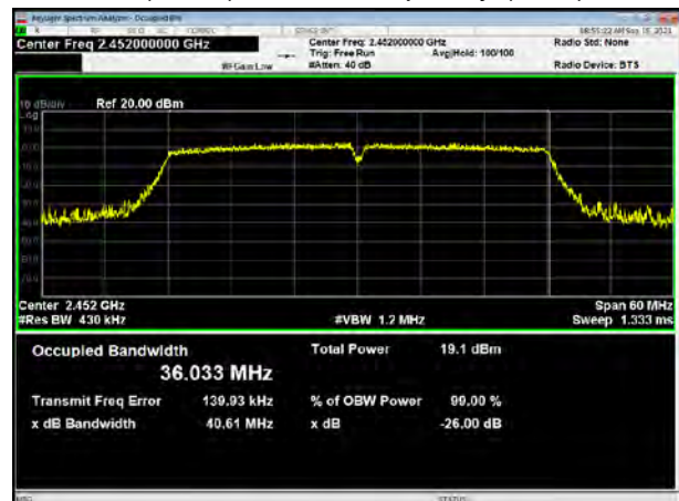
802.11n(HT40), Carrier frequency (MHz): 2452
