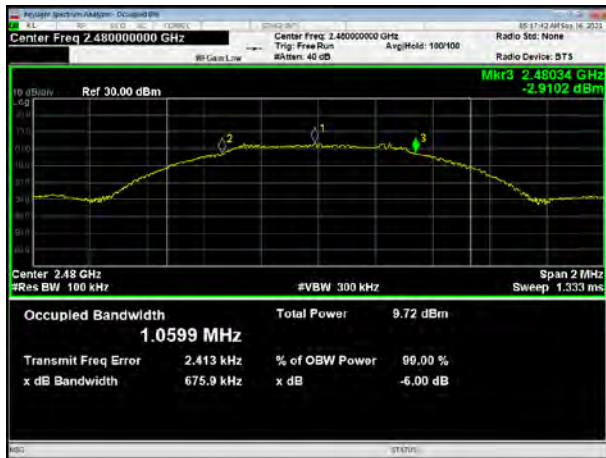
Bluetooth LE (1M) Carrier frequency (MHz): 2480
