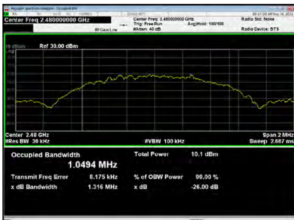
Bluetooth LE (1M) Carrier frequency (MHz): 2480
