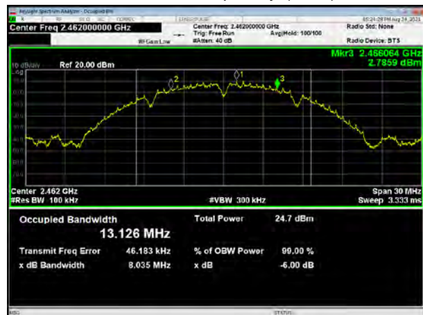
802.11b, Carrier frequency (MHz):2462
