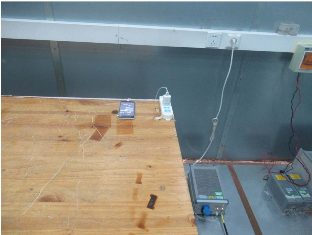
Picture 2 Conducted Emission Test Setup
