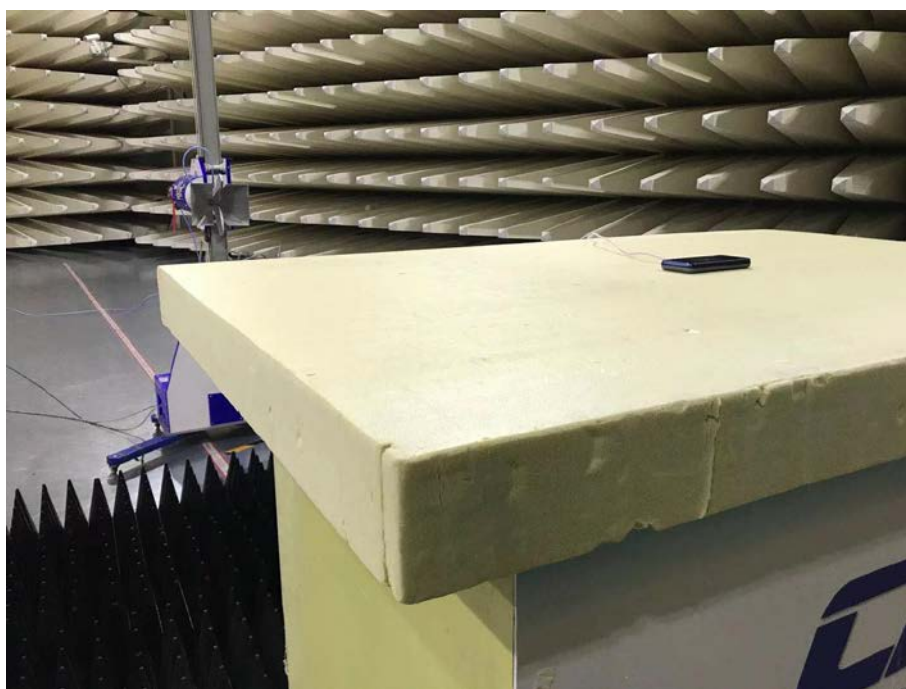
Spurious Radiated Emissions Test setup
