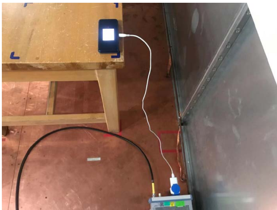
Conducted Emissions Test Setup (with charger)
